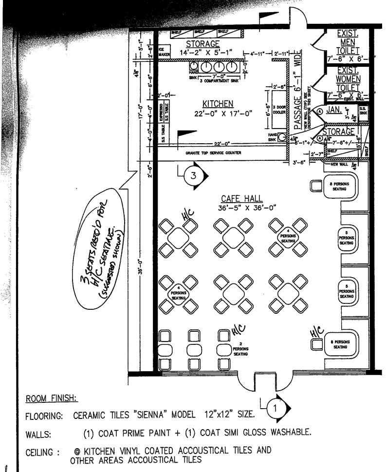
WALL BASE: CERAMIC TILE. PARTIAL FIRST FLOOR PLAN
