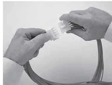
Logic Disconnect Plugs
