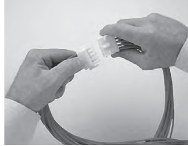
Logic Disconnect Plugs
