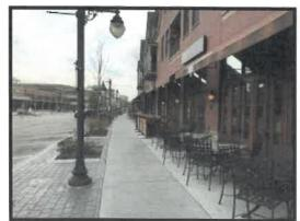
the pavers will be inlaid into the concrete surface to minimize future settlement of the pavers. The paver area will generally extend from the edge of the tree vaults to the curb line, as depicted in the above example image.
