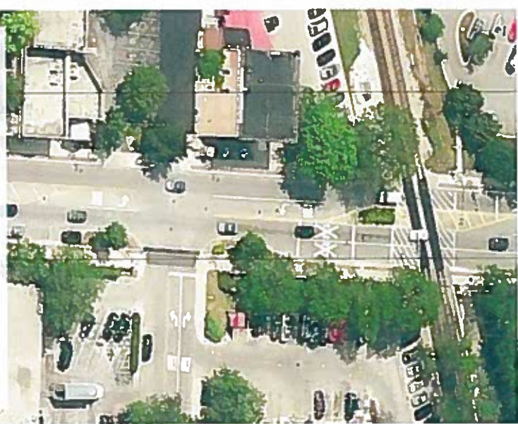
Glenview Road, Glenview, IL Glenview applied a road diet to the segment of Glenview Road that traverses through its downtown. The number of travel lanes reduced to 1 in each direction with a center lane for left-turns or handicapped medians. On-street parking is also provided.
