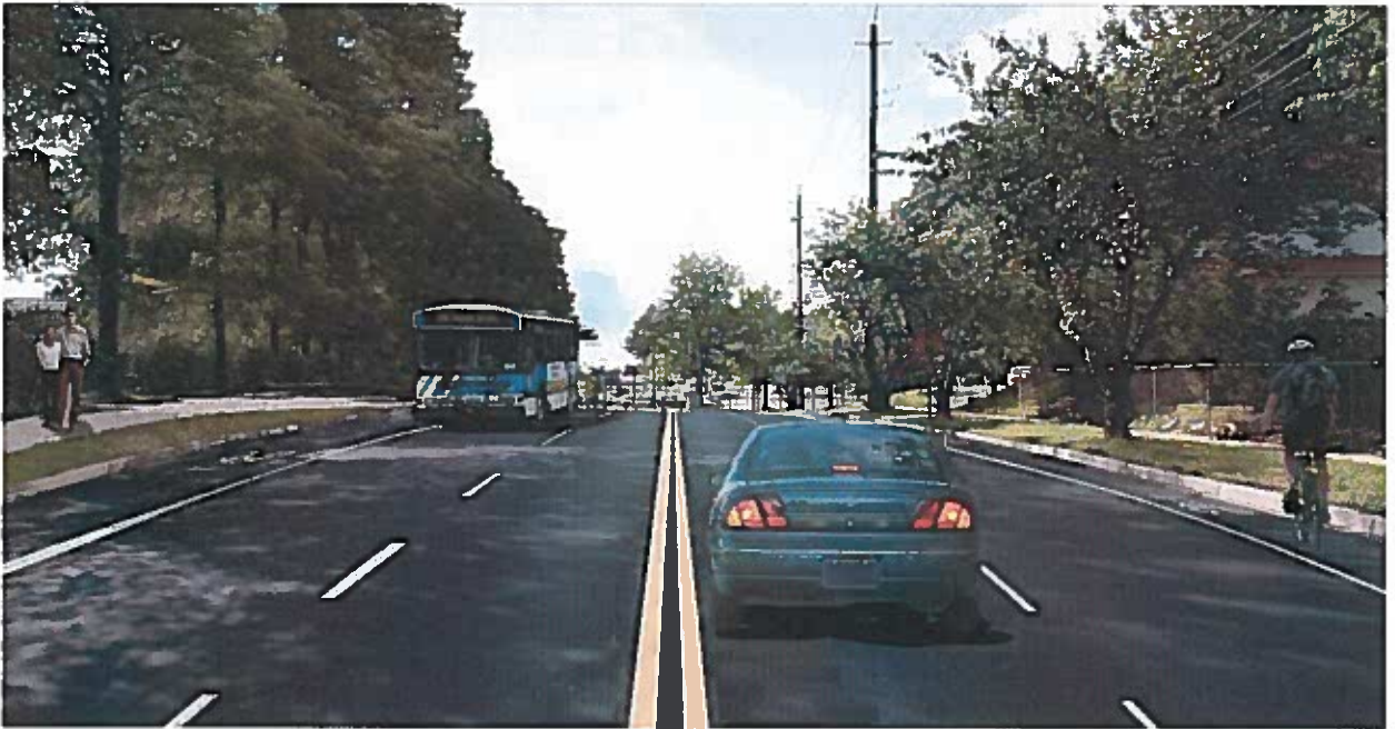
Example 2: Modifications include adding bicycle lanes and markings, a sidewalk with buffer, and pavement markings.
