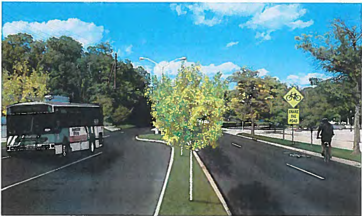
Example 3: Modifications include adding sidewalks with buffers, "Share the Road" signs, "sharrow" markings, and landscaping the median.
