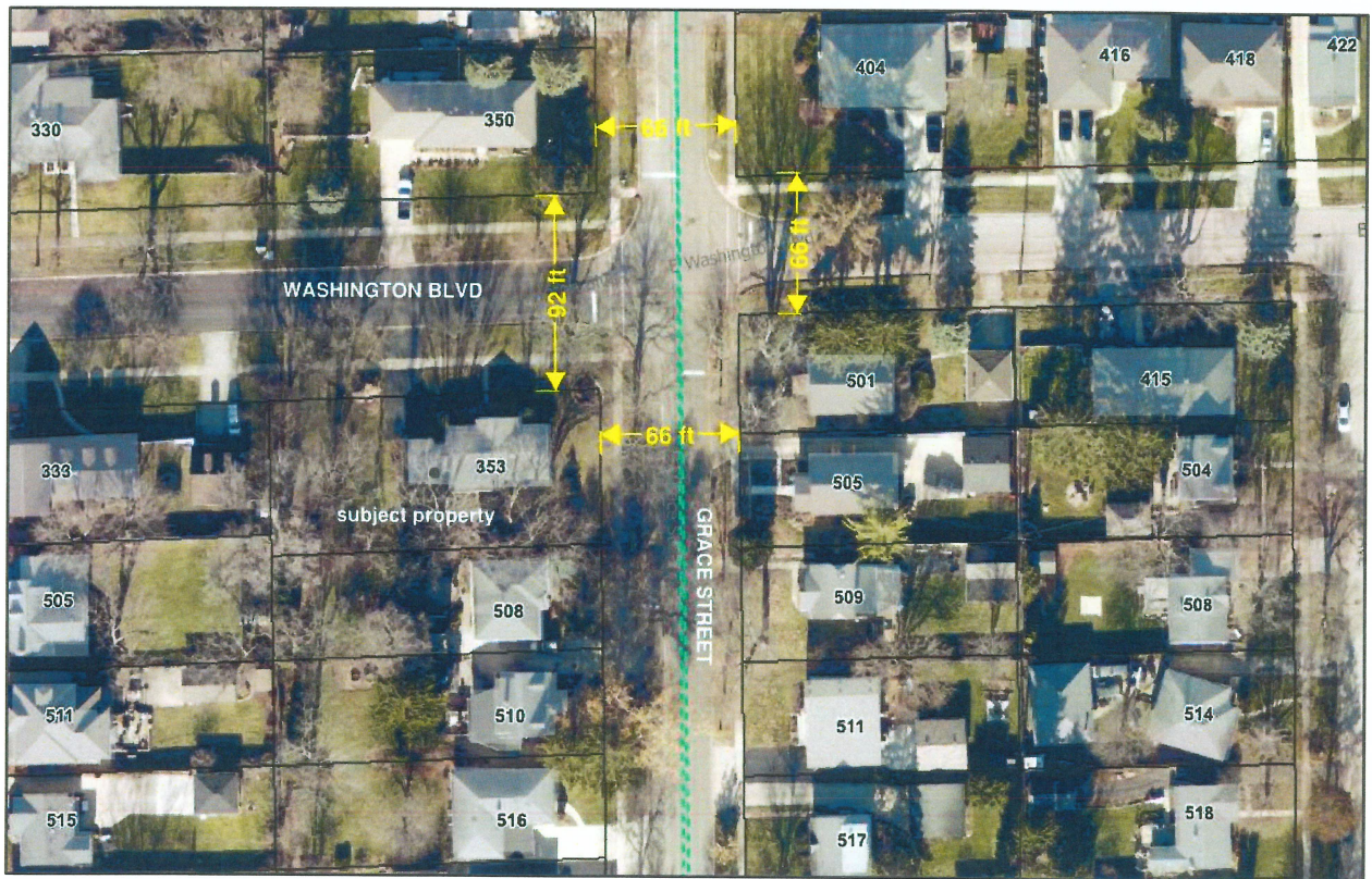
Figure 1. Right-of-way configuration in immediate neighborhood.
