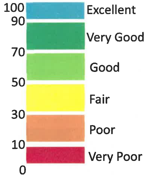
Figure 2: Typical Pavement Condition Index (PCI) Rating Scale
