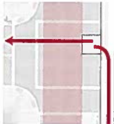
Cycle track turn box protected by physical buffer:
