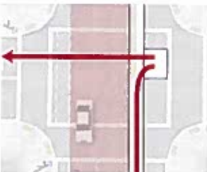
Bike lane turn box protected by parking lane:
