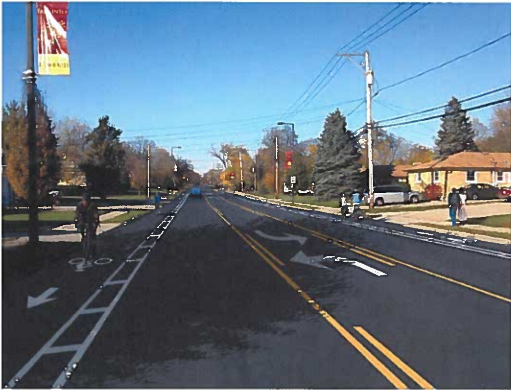
Figure 56. A photosimulation depicting Westmore-Meyers Road following a reallocation of travel lanes. The proposed design includes bike lanes and a center turn lane.
