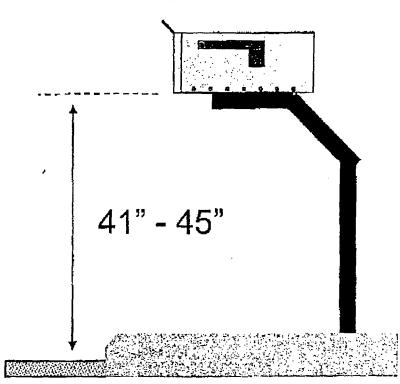
Generally, mailboxes are installed at a height of 41 to 45 inches from the road surface to the bottom of the mailbox.
