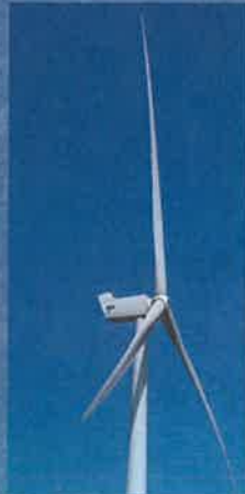
Horizontal Axis Turbine
