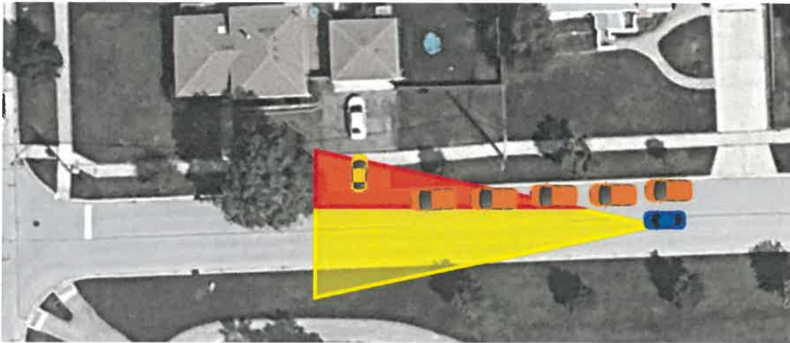
Illustration 1 – Limited visibility for drivers on Central Ave. to see cars backing out
